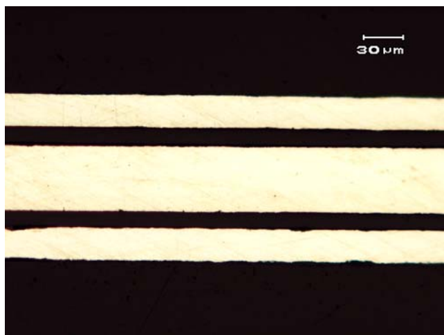
Fig. 2 Optical microscope image of a BME array in plan view containing a central, 50- \mu\text{m} -wide Al–40% Zn alloy band flanked by two 25- \mu\text{m} -wide Zn bands, separated by 10 \mu\text{m}
